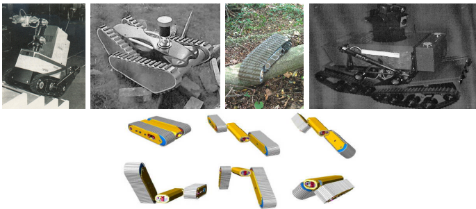
Fig. 2. Variable tracked configuration robots [16]: Pandora [17], AURORA [18], link-type tracked vehicle [25], and NUGV [26]
