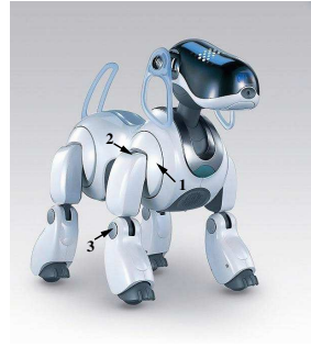
Fig. 1. A Sony Aibo ERS-7. The arrows point to the shoulder (1), abductor (2), and knee joint (3) of the Aibo's right front leg.
