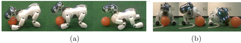
Fig. 1. (a) Representation of FALL-KICK from left to right (b) Representation of HEAD-KICK from left to right
