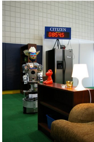
Fig. 1. Robot TPR8, this robot has, for sensing the environment, a ring of sonars, a laser measurement system, a microphone and a vision system
