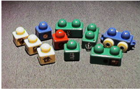
Fig. 3. The complete set of Electronic Blocks. The sensor blocks are to the left, the logic blocks are in the centre and the action blocks to the right.
